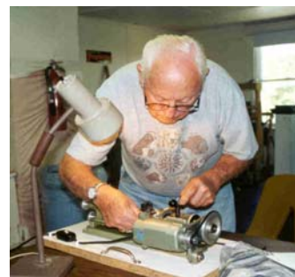
David Barnes is making pivot holders for polish-pivots on the lathe.
