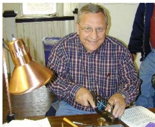
Ron Oorlog is cutting a brass plug to be soldered in a spring barrel for the Spring Barrel Class 200.
