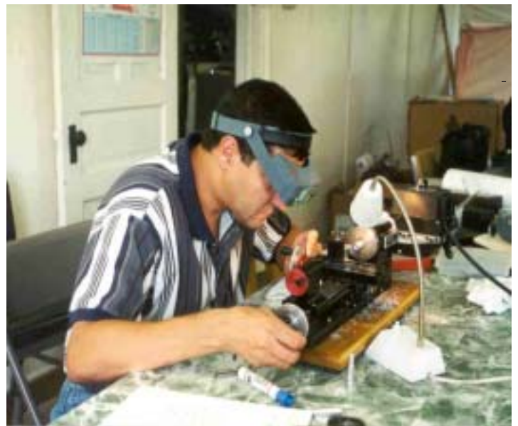
This photo is of Alex Santa-Pinter using a Sherline lathe to work on his first project. The students were given blank tool cutters and they ground them to use on the projects. The first project was making a tool for removing the spindle in a jeweler's lathe out of aluminum.
